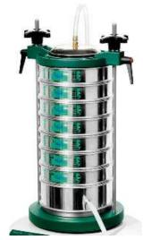
The O-ring seals are fitted on to the outside of the bottom rim of each sieve, which means the sieves are stacked onto each other and they form a seal.
