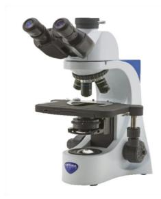
Trinocular brightfield microscope, 1000x, IOS N-PLAN objectives
