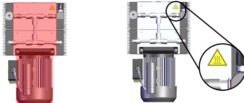
Fig. 2-1 Hot zone on the device, warning label Top view (right)
