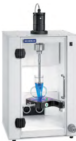
Configuration example LS 20 for direct sonication
