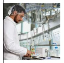
Measure density near production line: The new measuring cell design minimizes the influence of external mechanical vibrations and allows for precise results even in turbulent environments.
