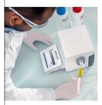
Measure density, refractive index as well as many related values, such as specific gravity, % alcohol, or Brix of your samples quickly and reliably. No need for table lookup or conversions: the instrument performs all necessary calculations. Green, go. Red, stop
