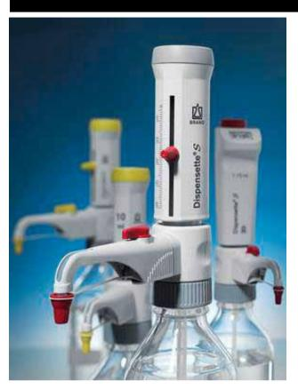
The New Generation Dispensette®S with its broad range of application has proven reliable for accurate dispensing even of aggressive reagents.
