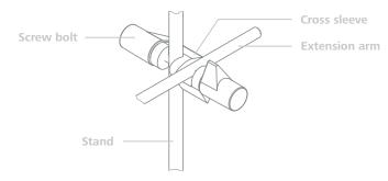
Check that the stirrer is held in position firmly prior to each use and also at regular intervals. The position of the stirrer must only be adjusted when the equipment is stationary and the power supply is disconnected.
