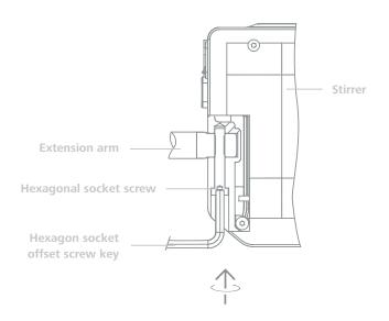
Ensure that the extension arm is fitted securely.
