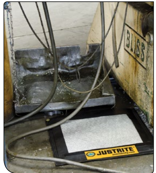
Position drip pad in tight spaces between machinery to capture oily leaks.
