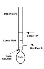
**Assembly:** Attach rubber tubing to the side-arm of the Bubble Flowmeter. Fill the bulb with soap solution (water and detergent, or Snoop®) and attach to the bottom of the Bubble Flowmeter. Mount the Bubble Flowmeter near the gas supply to be measured, then attach the tubing to the gas supply.
