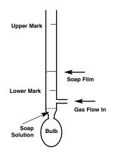
**Assembly:** Attach rubber tubing to the side-arm of the Bubble Flowmeter. Fill the bulb with soap solution (water and detergent, or Snoop®) and attach to the bottom of the Bubble Flowmeter. Mount the Bubble Flowmeter near the gas supply to be measured, then attach the tubing to the gas supply.
